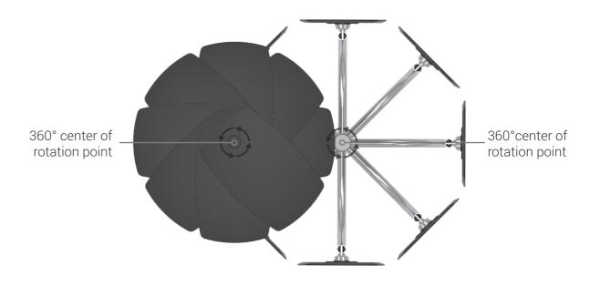
The 360° table and pipe, allows the user to find the perfect position when using the Easy. When stowed away, it can be moved around out of the way. Images can be found on pages 6-7 showing the Easy in various positions on the Ned Pringle Chair.
